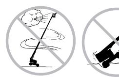
Use extreme care and slow speeds while driving the machine in the stowed position across uneven terrain, debris, unstable or slippery surfaces and near holes and drop-offs. Do not drive the machine on or near uneven terrain, unstable surfaces or other hazardous conditions with the boom raised or extended.
